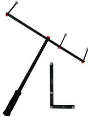
Figure 2: Tools for calibration: Wand and L-frame [1, p.104]
