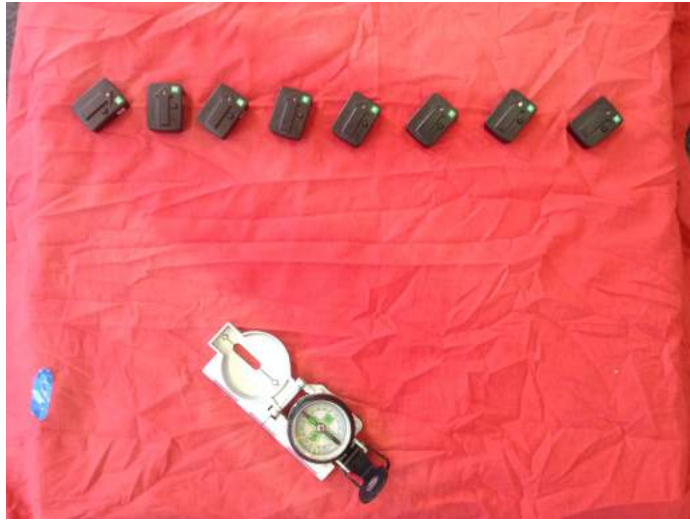
Figure 7: Different Offsets in z-direction: IMUs (black) point towards different north-poles while compass (grey) shows actual north-pole
