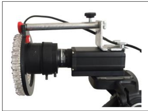
Figure 1: Lens and ringlight mounted on the camera. 23
