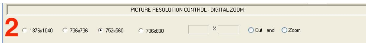
This box controls the resolution of pictures of a recording or single picture taken. Left are some preset sizes. 1376x1040 is the full resolution of the camera.
